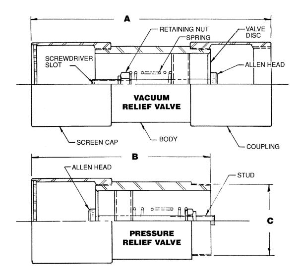
To adjust Vacuum or Pressure Relief Valve, remove Screen Cap, hold Retaining Nut or Allen Head with Wrench and turn stud with screwdriver. It is suggested that a vacuum or pressure gauge be used to make accurate adjustments.
